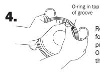
Roll your thumbs back and forth over the O-ring while pushing upward until the O-ring falls into the top of the groove.
