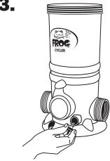
Unscrew knob from the front of POOL FROG Cycler. Allow all water to drain.
