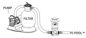
The POOL FROG Cycler should always be installed between the filter and pool (or between heater and pool if applicable). Never install POOL FROG Cycler before the heater or damage to the heater could occur.
