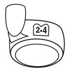
After each testing, adjust the dial up by 1/2 increment if the free chlorine reading has dropped below 0.5 ppm or adjust down by 1/2 increment if the reading has risen above 1.0 ppm. Continue this process each day until the free chlorine reading stabilizes to at least 0.5 ppm.
