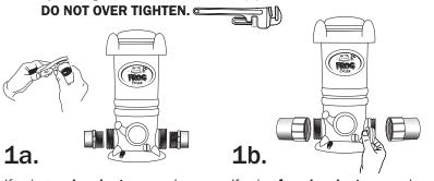
If using **male adapters**, apply pipe thread tape or sealant to the threaded end of each adapter.
