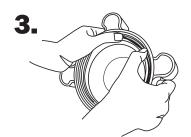
Place your thumbs on each side of the cap over the O-ring in the groove.
