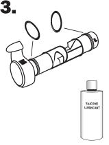
Replace both O-rings. Apply silicone lubricant that came with your POOL FROG Cycler on O-rings.
