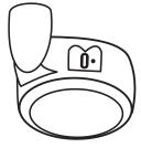
Turn off pump and turn control dial to Setting 0. This reduces the flow of water into the unit when the cap is open.
