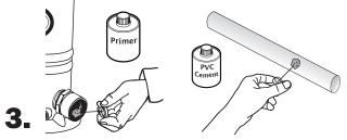
Following Primer directions, brush Primer on the inside of the adapters and to ends of pipe. Repeat this process with PVC cement following manufacturer's directions on that product.
