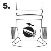
Replace locking pin by pushing it through the slots on the dial until it locks into place.
