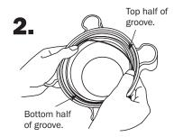
Place new O-ring in bottom half of groove.
