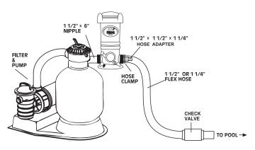
To prevent damage to heaters or filters, see your dealer about installing a **corrosion resistant** check valve which will reduce the back flow of chlorine gas when the Cycler is turned off.
