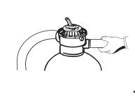
Screw one end of nipple into the filter return. Hand tighten. Finish tightening by turning 1 to 2 revolutions with a pipe wrench.
