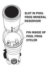
Find slot on side of POOL FROG Mineral Reservoir and line up with fin inside the POOL FROG Cycler. Lower POOL FROG Mineral Reservoir into POOL FROG Cycler until
